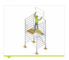
8<sup>th</sup> STAGE Place 1 diagonal and a Guardrail from the working platforms.
