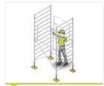
**6<sup>th</sup> STAGE**Place another 2 elements and then close the Guardrail safety latch.
