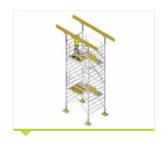
**15**th **STAGE**Place the beams on the forks.
