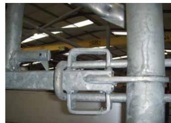
The Towrok® shoring system can be easily adapted to any kind of formwork.
