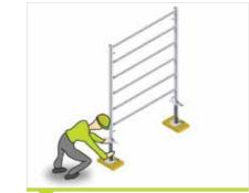
Assemble 2 base levellers and then the shoring element.
