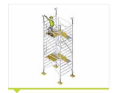
**14<sup>th</sup> STAGE**Assemble the forks and adjust to the necessary elevation.
